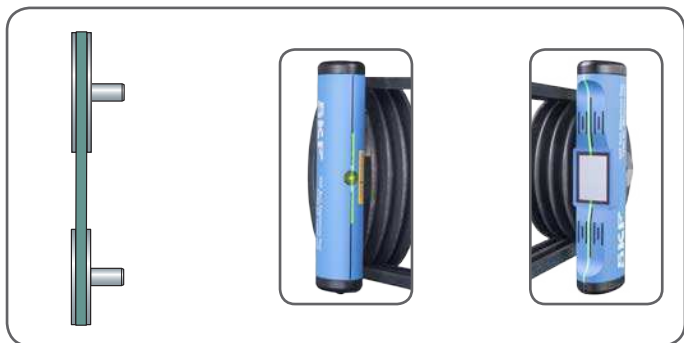
Figure 9 Pulleys perfectly aligned
